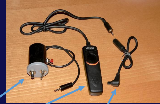
Homemade bulb controller Standard bulb controller Adapter cable: jack to N3
